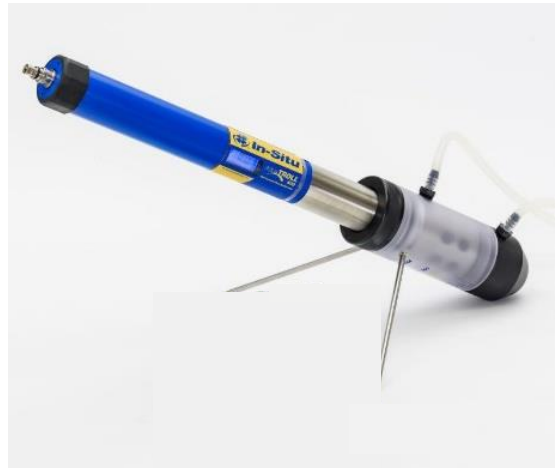
Aqua TROLL 600 z systemem Low-Flow sampling
